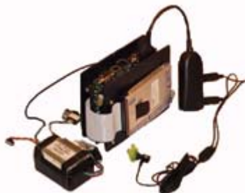
COMOTION prototype portable unit: personal computer, GPS receiver, wireless modem, earphone, and microphone
